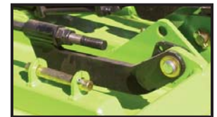
Floating hitch eliminates stress on frame
