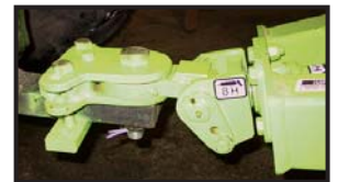
Optional precision hitch eliminates drawbar wear & spreads drawbar weight more evenly
