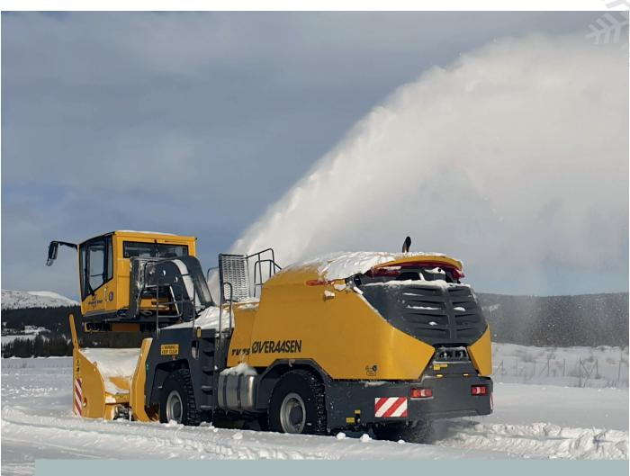
The ØVERAASEN TV 750 Performance Line is a new self-propelled snowblower, which is the smallest of the big snowblowers from Øveraasen. The TV 750 has a clearing capacity of 6 500 tons/h / 7 165 US tons/h at a casting distance of 25 m / 82 ft, and with this it rounds off the portfolio of applications for the medium performance segment. The high transport and operating speed makes it possible to carry out the snow clearing reliably and safely in the predefined time window.
