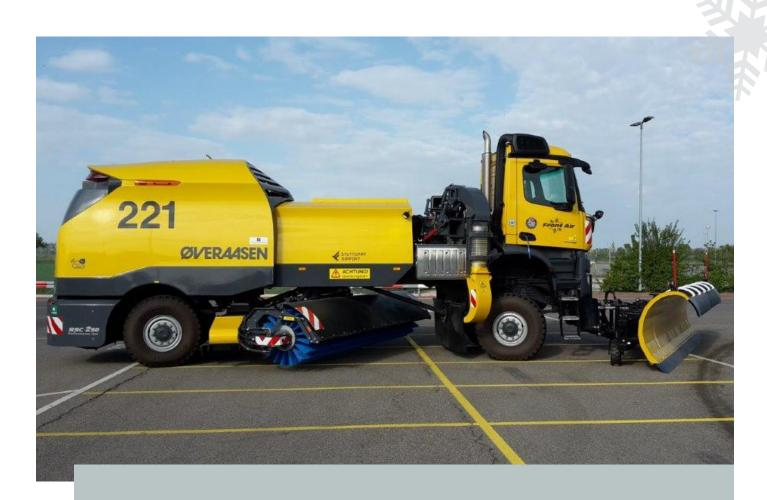
The ØVERAASEN RSC 250 Performance Line is designed for use on runways, taxiways and narrow apron areas; the RSC 250 offers the highest degree of maneuverability and clearing performance. The largest advantage of the ØVERAASEN RSC 250 is the vehicle and its compact design. This makes the ØVERAASEN RSC 250 unique for the market for unrestricted use, even on runways without influence on the snow clearing result.
