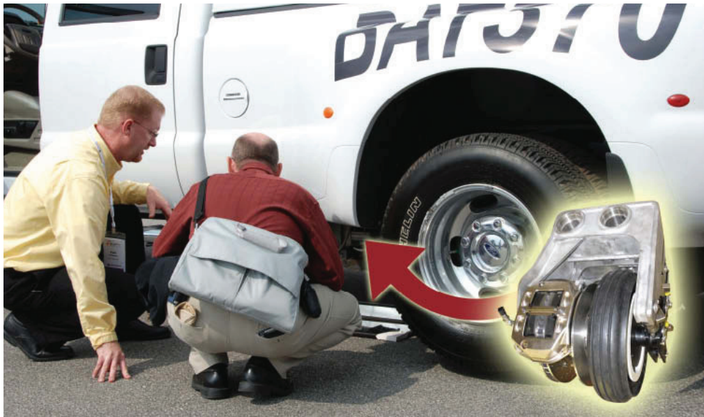
This Braking Availability Prototype Test Vehicle, developed by the University of Waterloo and Team Eagle, will be tested this winter by the Region of Waterloo International Airport and WestJet. It mimics the wheel braking characteristics of a braking aircraft and provides realistic values that can be used by pilots to predict the wheel-braking performance of their aircraft.
