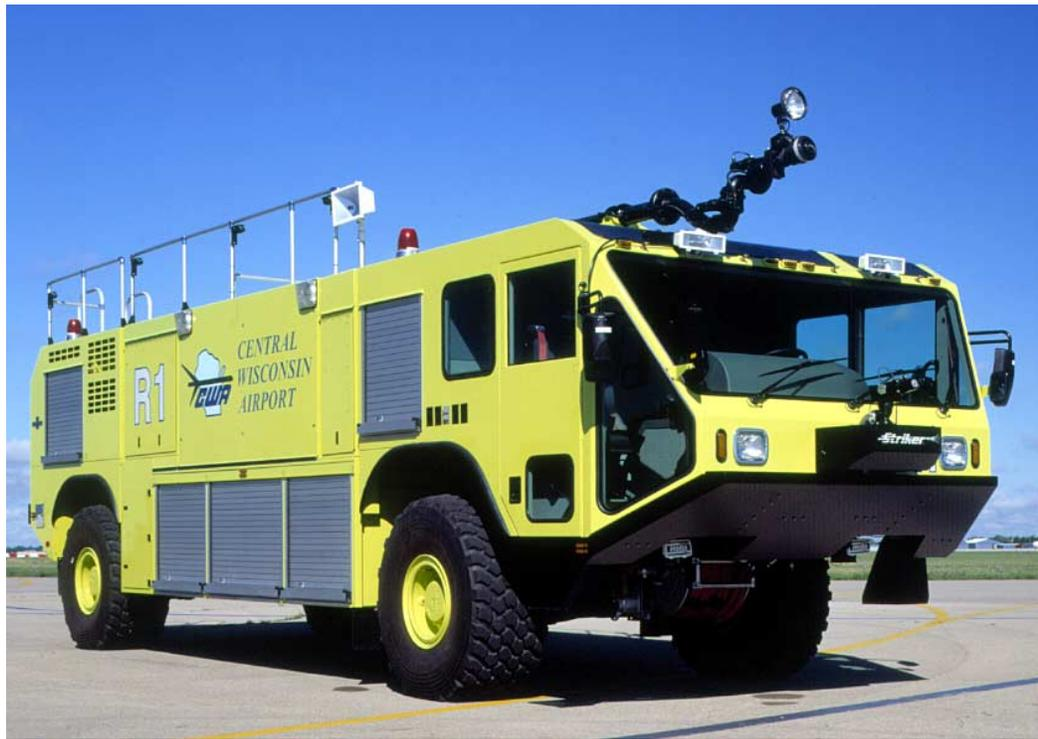
**EXTREME MOBILITY.** Your response doesn't stop where the runway ends. With all-wheel drive and Oshkosh TAK-4™ independent suspension as standard features, the Striker can outmaneuver and outperform any ARFF vehicle in its class on and off the runway. The unique independent suspension system reduces stopping distance and helps tires hug the pavement for enhanced cornering and handling. Ground clearance is a full 17 inches (43.2 cm).
